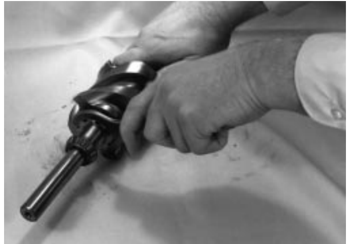
Fig.7. Centering cam on shaft
