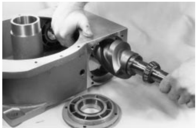
Fig. 5 Removing input shaft assembly
