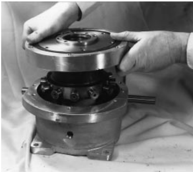
Fig.1 Output shaft removal
