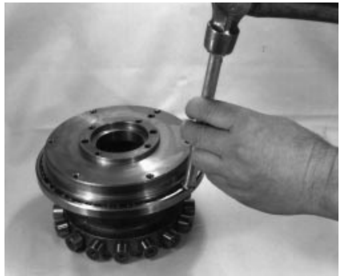
Fig .4. Removing output bearing.
