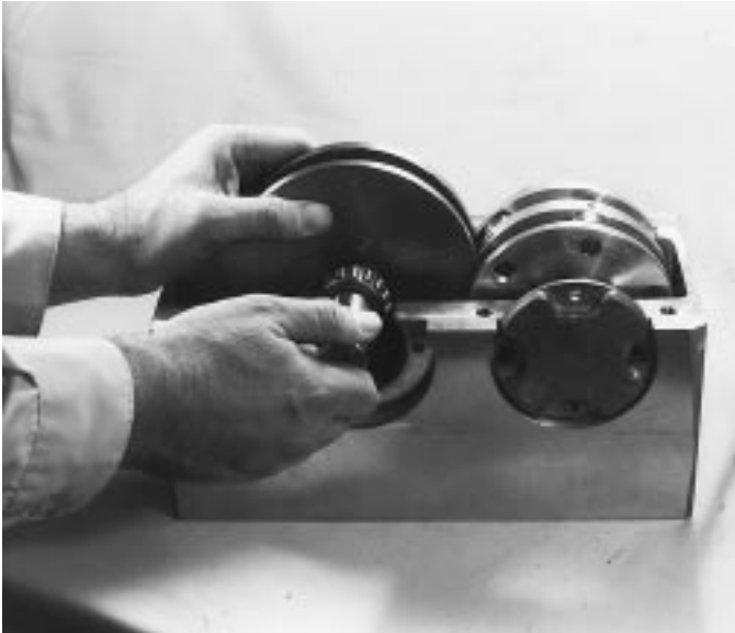
Fig.4 Removing input shaft.
