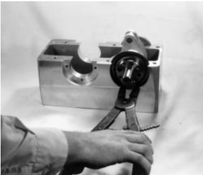
Fig.5 Removing snap ring.
