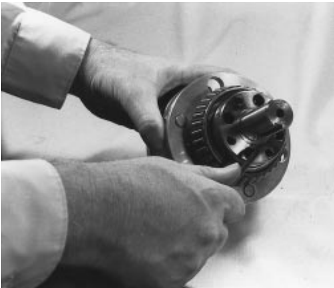
Fig.6 Removing follower wheel fasteners.
