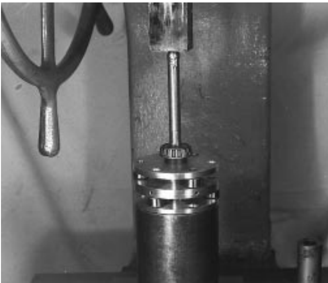
Fig.7.1 Pressing out shaft.
