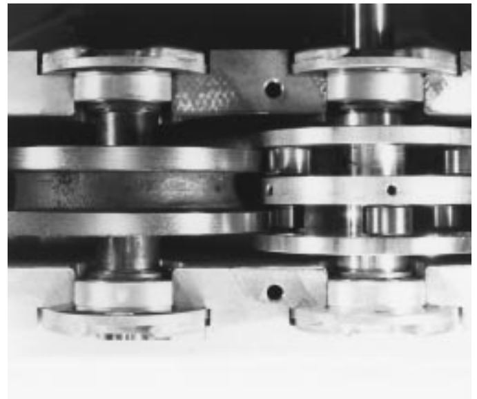
Fig.9 Cams preloaded against followers.
